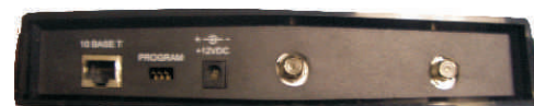
Back panel with 10 Base T, Programming output, 12VDC plug and Antenna posts
